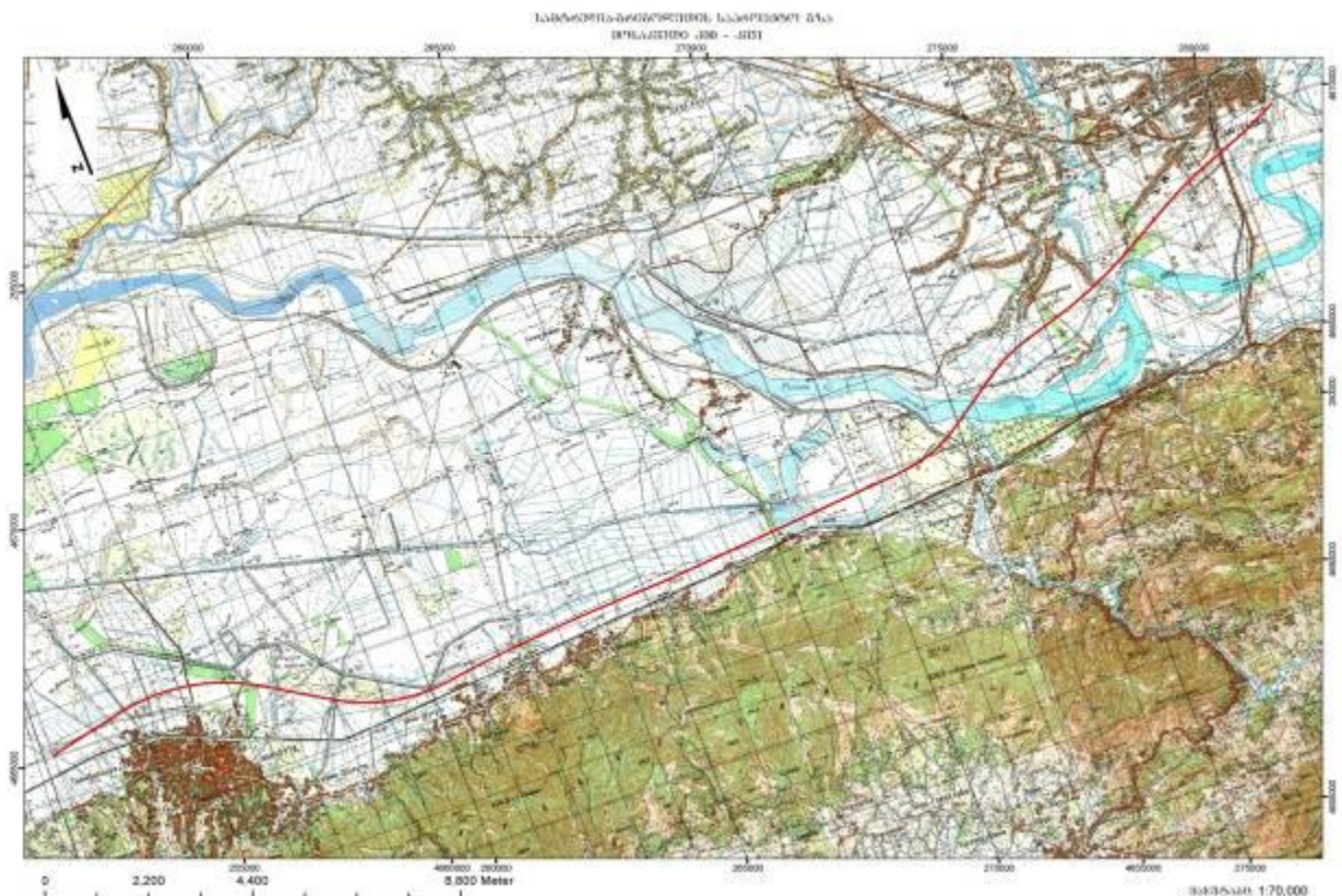
Fig. 4.7. Location of the geomorphologic elements and hydrographic network of the design road, Samtredia-Lanchkhuti section of the modernization road and its adjacent area. The red line marks the design road (topo-base scale: 1:70 000)
