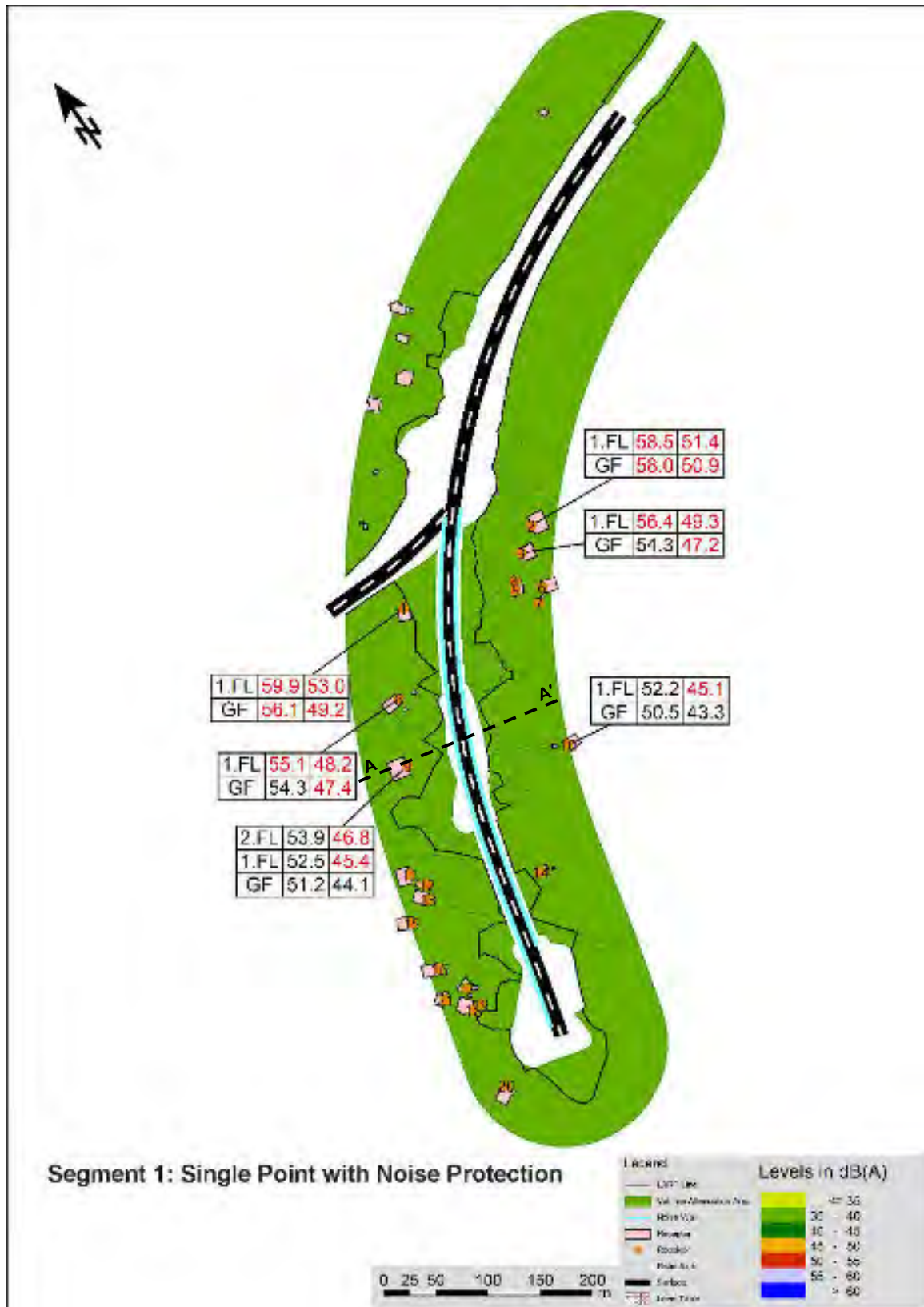
Figure 8-32: Segment 1-Single Point with Noise Protection
