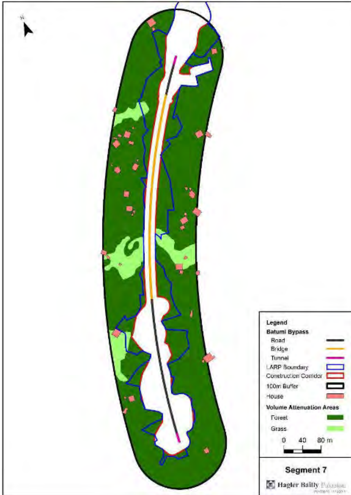
Figure 8-23: Segment 7 Noise Modeling
