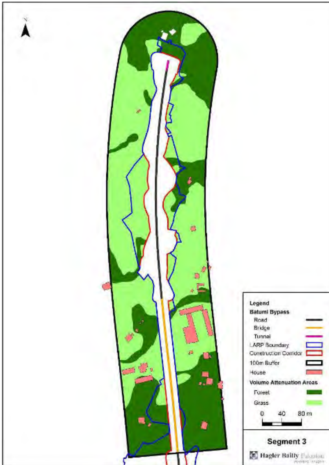
Figure 8-11: Segment 3 Noise Modeling
