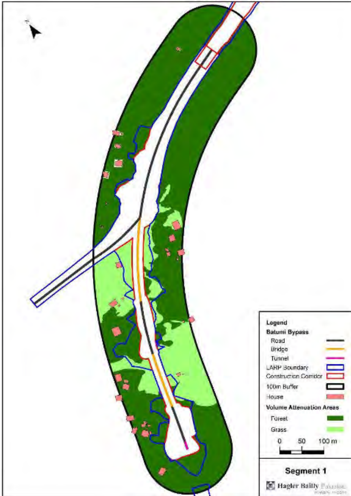
Figure 8-5: Segment 1 Noise Modeling
