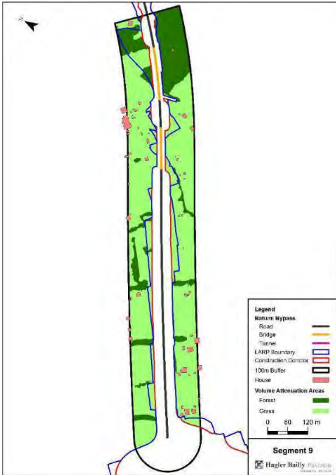
Figure 8-29: Segment 9 Noise Modeling
