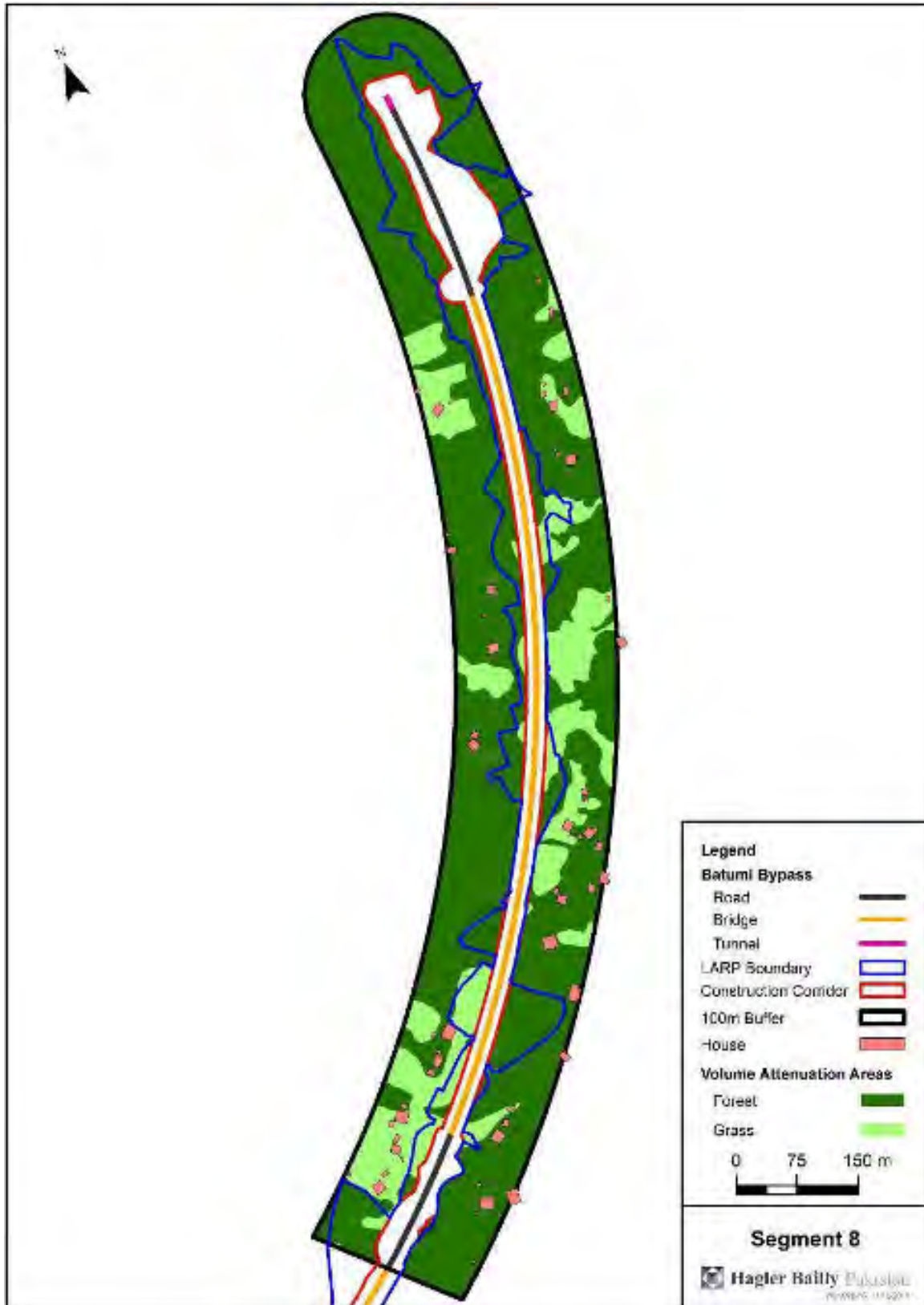
Figure 8-26: Segment 8 Noise Modeling
