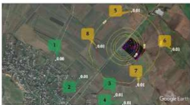
Maximum concentration of insecticide total impact group 6009 (index 301-330) at control points (nos. 1-4), at the nearest settlements and at the border of 500-m radii zone (nos. 5-8)
