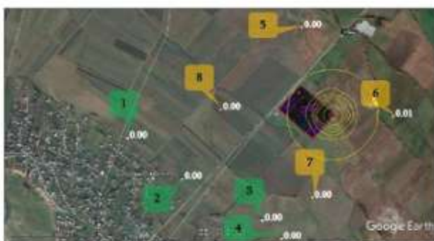
Maximum concentration of heavy fractions of saturated hydrocarbon (code 2734) at control points (nos. 1-4), at the nearest settlements and at the border of 500-m radii zone (nos. 5-8).
