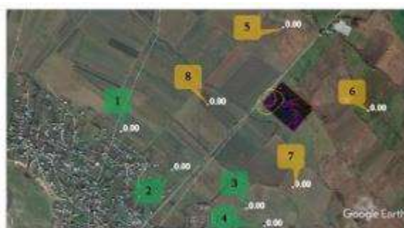
Maximum concentration of nitrogen oxide (code 324) at control points (nos. 1-4), at the nearest settlements and at the border of 500-m radii zone (nos. 5-8).
