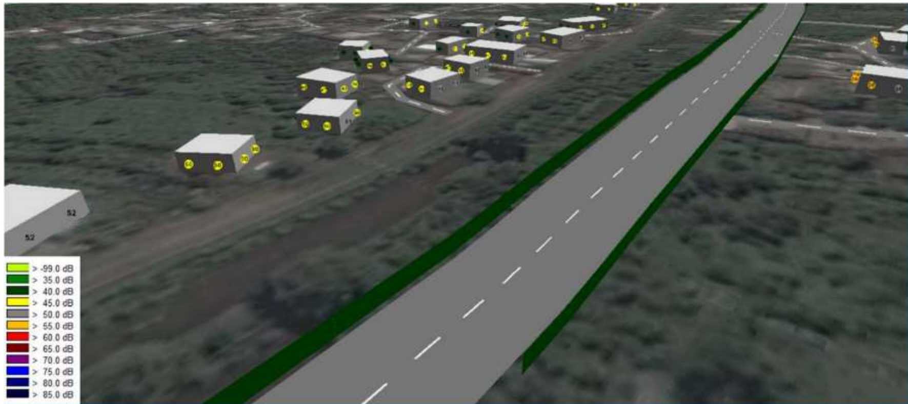
Figure 7.3.5.2.: Noise level by using barriers by 2025 (Vilage Kirovka)
