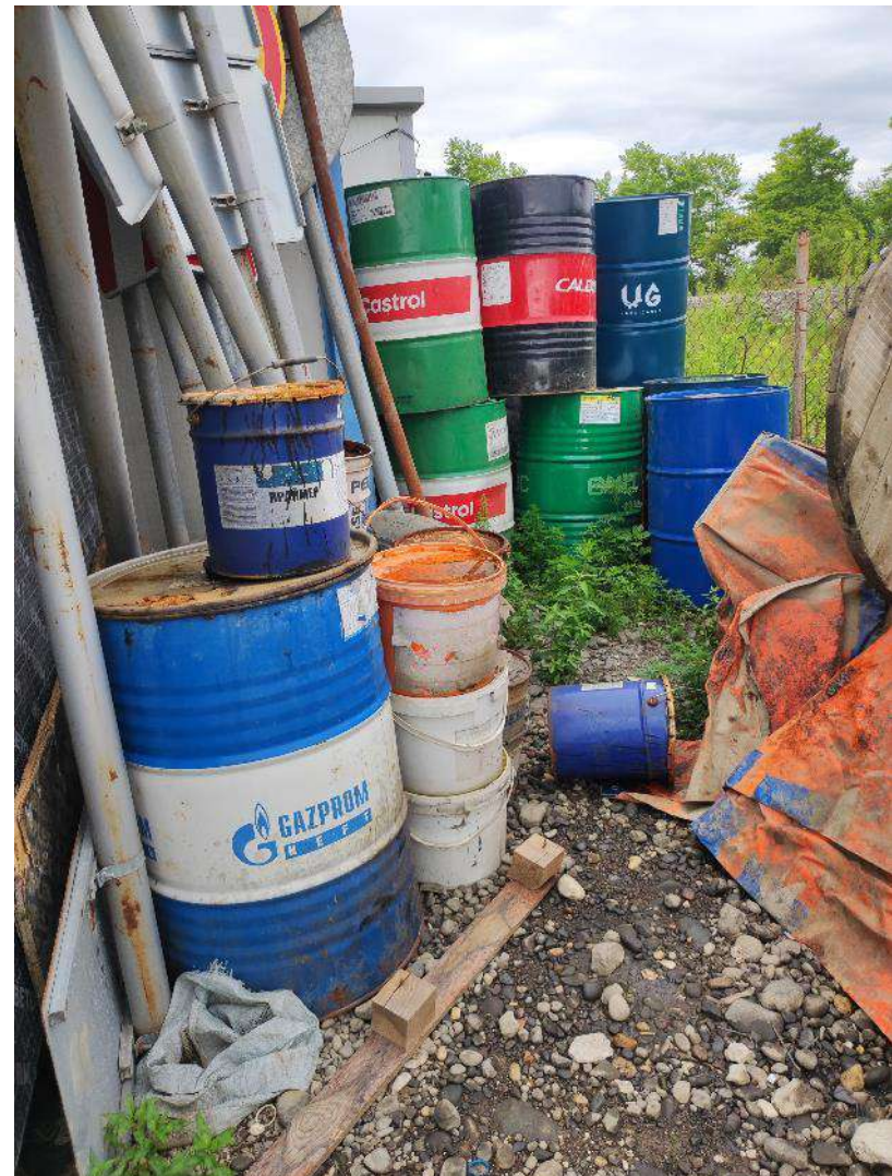
Improperly stored hazardous waste
