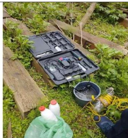
Fig. 4.1.4 - Multiparameter Water Quality Meter
