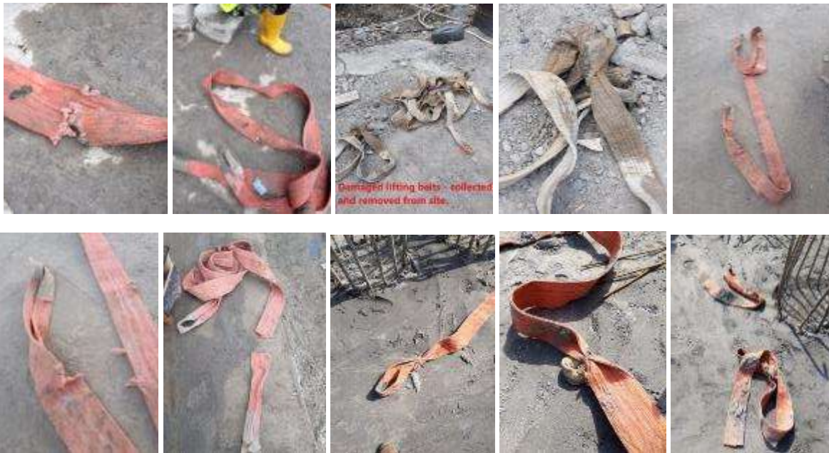
Picture 3: Non-compliance (Damaged lifting equipment) (All tunnels): - Damaged and cut lifting equipment has been found at workplaces during visiting the tunnels. Site responsible persons from the Contractor Company were informed about it by the Engineer. The Engineer has asked Contractor to pay additional attention to the workplace safety and do inspection of using tools and equipment (Including lifting equipment) very often for to find and remove from the site all damaged or cut equipment. Three of such damaged lifting belts has been found by the Engineer and cut it in pieces to avoid further usage and any type of possible incidents from happening. Issue closed.
