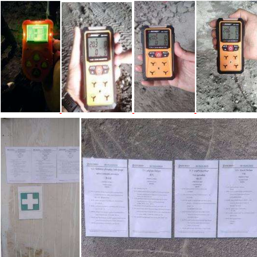
Picture 23: Good observation (Compliance to work process) Tunnel №2 AT, Tunnel №5 AT and TA - Information about the air concentration norms are placed at the entrances of the each tunnels. All the tunnels are equipped with air/gas measuring equipment and air concentration levels in the tunnel is under regularly monitoring (During the specific works in the tunnel air must be systematically monitored and the information must be recorded). Air/Gas Detectors have been tested and they were in working order. A bump test involves exposing the detector's sensors to a concentration of gas that is greater than the alarm set points. During the testing, level of CO was checked up inside the tunnel, and detected increased concentration of CO. It started to flash in red color. Issue closed.
