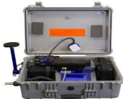
Figure 3-1 Dust Monitoring equipment
