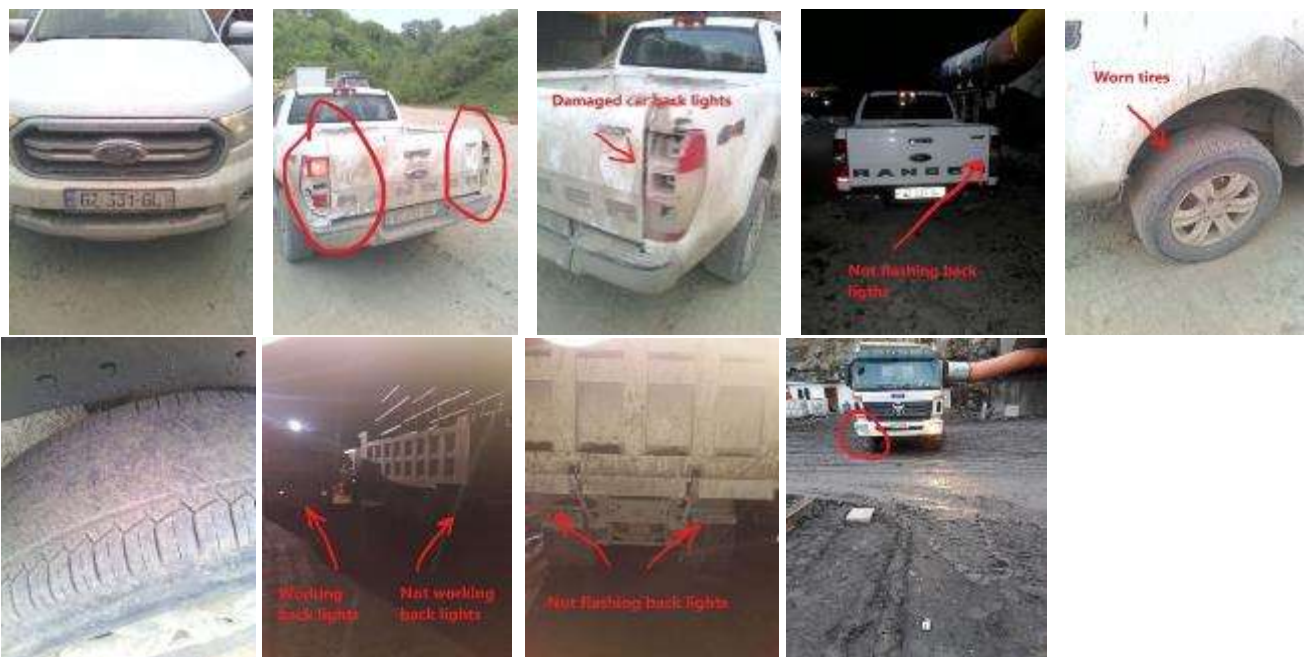
Picture 4: Non-compliance (Driving safety): Continue non-compliance to international H&S rules and requirement has been observed during site walk. More vehicles and trucks with damaged traffic lights and worn
