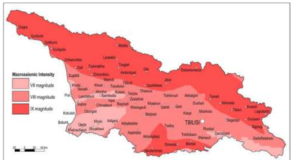
Figure 6.14. Seismic intensiveness map of Georgia (Source: Construction norms and rules – Aseismic stable construction, pn 36.0101-09)
