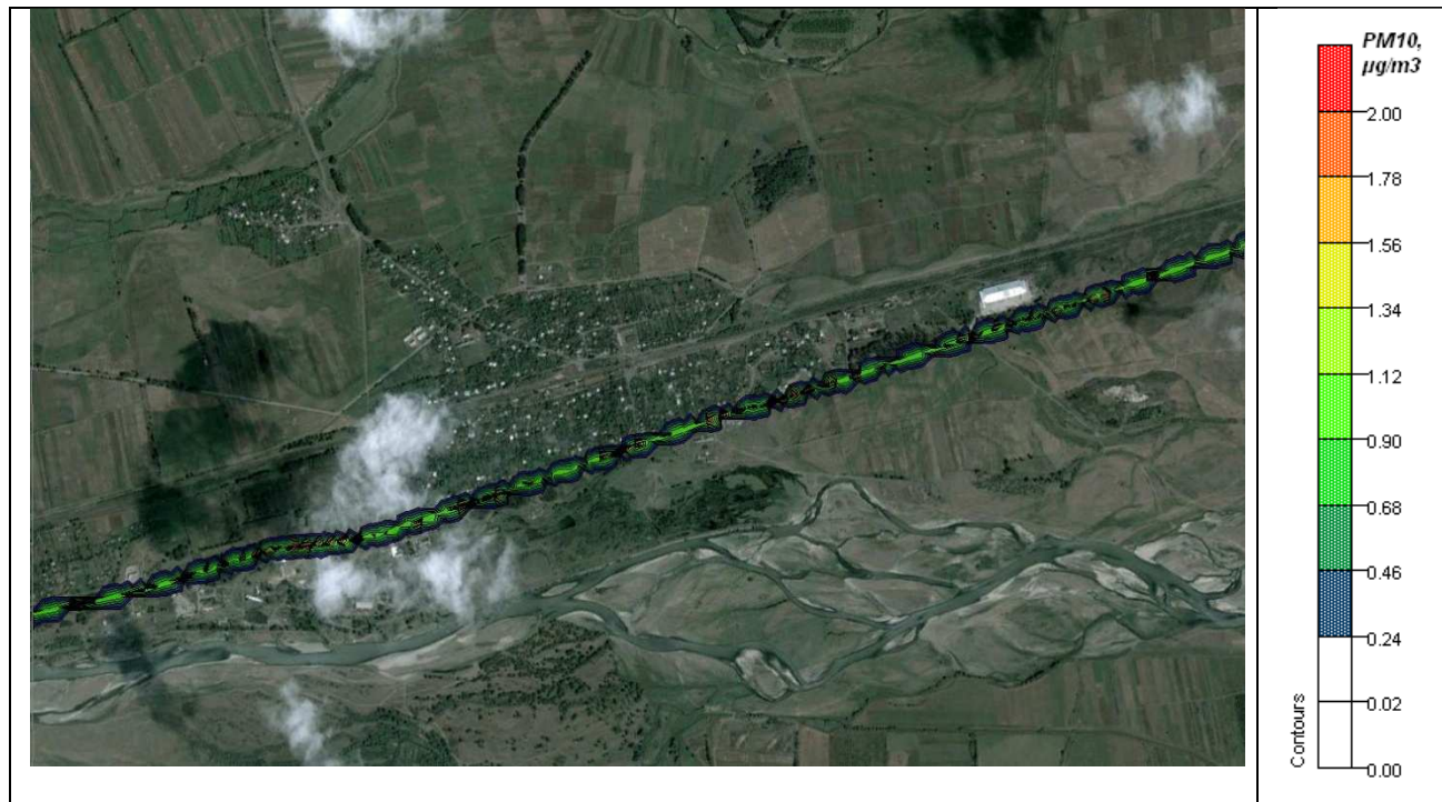
Figure 15 PM 10 dispersion* along E-60 EWH section between Agara and Didi Sative, 115 - 121 km of the existing road, "Zero" alternative
